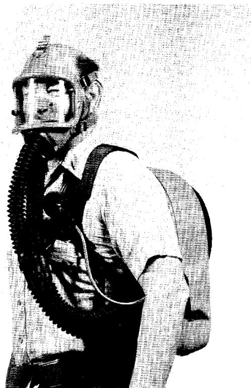
In this closed-circuit, self-contained breathing apparatus, air is supplied from the back-carried unit through one of the tubes to the mask. The exhaled air returns through the other tube to the back unit for cleaning, restoration to breathing quality and recirculation. LASL tests such respirators and makes recommendations to the NRC
